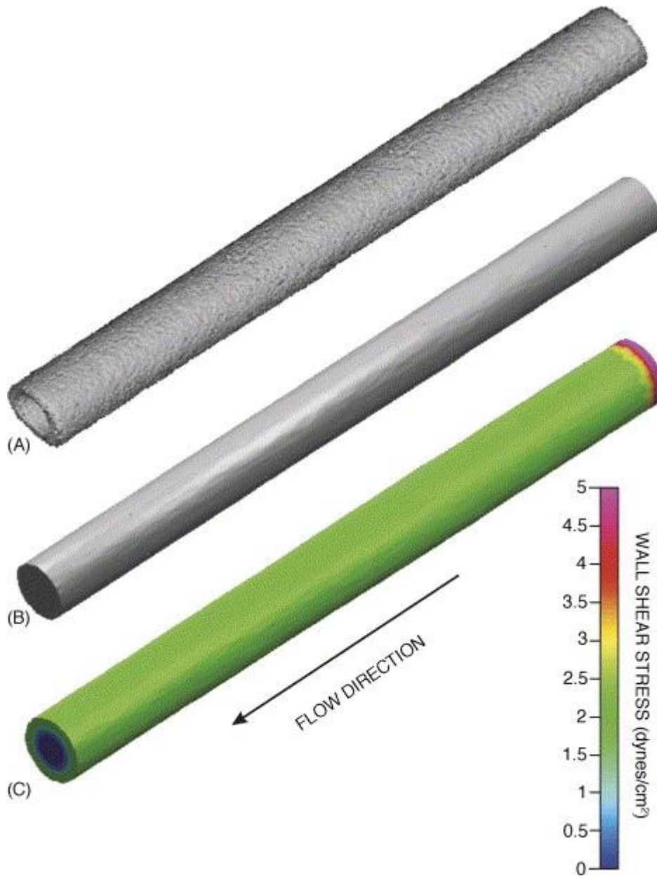
Fig. 8. Surface smoothing of a reconstructed polyethylene tube. Illustrations of a rendered polyethylene tube obtained before (A) and after (B) implementation of the surface smoothing operations discussed in the text. The uniformity of WSS distributions along the wall of the reconstructed and smoothed polyethylene tube is depicted in (C).
