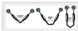
Figure 1. Expected geometries for metals (M) binding to tethered monodentate heterocycles with unspecified Lewis donor atoms (black spheres) containing one-atom (left), two-atom (center), and three-atom spacers (right).
