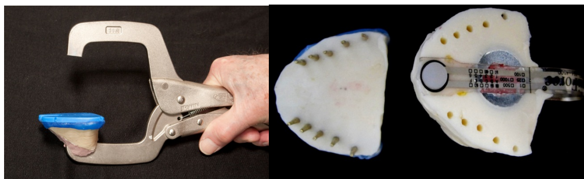
778 779 Figure 13. Illustrates the mounting jig on the left. The upper mounting base in 780 the center showing the dowels permitting the vertical travel, yet maintaining the 781 inter-arch relationship of the models. On the right, a FlexiForce® sensor is 782 shown inserted directly over the anterior teeth.
