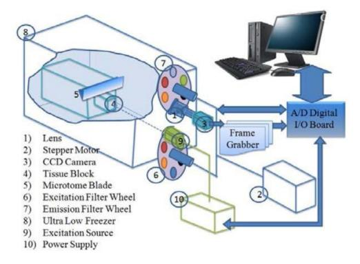
Fig. 1 Schematic of cryoimager.<sup>33</sup>
