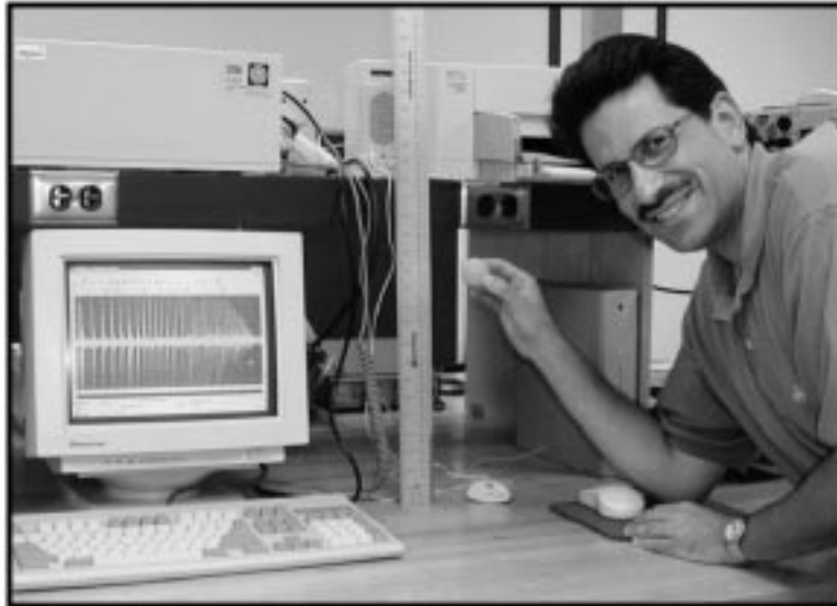
Fig. 1. Photograph of experimental setup (ball to be dropped in front of microphone).
