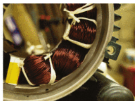
(a) Winding process of the randomly wound 12-slot 10-pole machine
