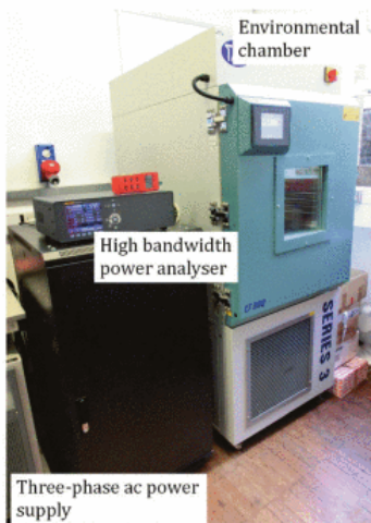
(b) Experimental setup used for measurement of ac winding losses
