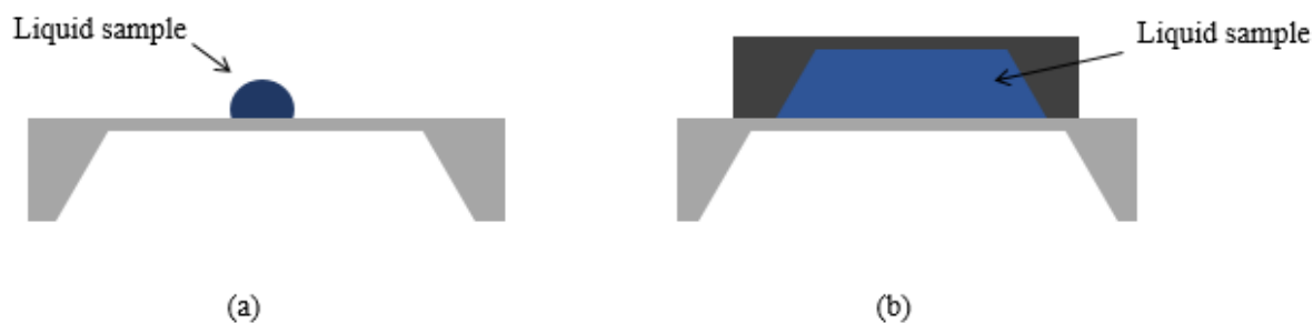
Figure 3-1 Sectional view of open chamber calorimeter (a) and closed chamber calorimeter (b).
