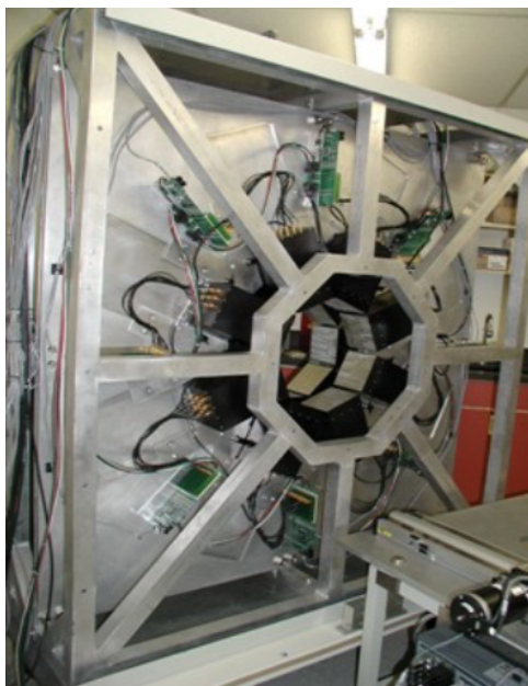
Figure 2.12: Picture of the FastSPECT II system with the outer shielding removed, revealing the gamma camera arrangement [54].
