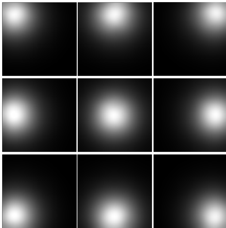
Figure A.3: In situ mean response of each of the 9 PMTs to a well collimated point source positioned on a 78 x 78 grid in front of the camera (based on figure 12.2 in [21]).
