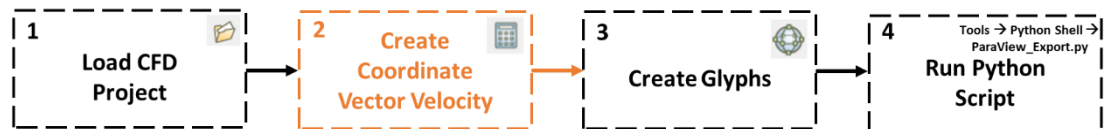
Figure 21: Flowchart to create 3D geometry velocity glyph files (.vrml). Icons on the top right corner of steps 1-3 represent: (1) open, (2) calculator, (3) glyph. Step 2 can be skipped depending on the CFD file
