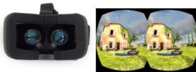
Figure 10: Left- Oculus Rift, with its wide-angle lenses. Right- input for HMD [46]
