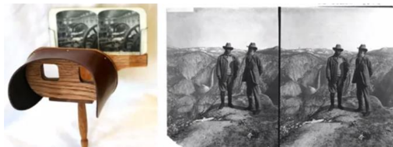
Figure 8: Stereoscope using stereovision [42]
