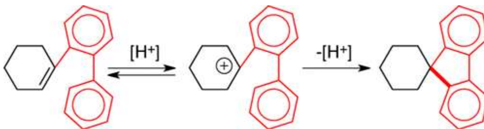
Scheme 1. Example of Intramolecular Friedel–Crafts Reaction to Construct Fluorenylcyclohexane Ring System
