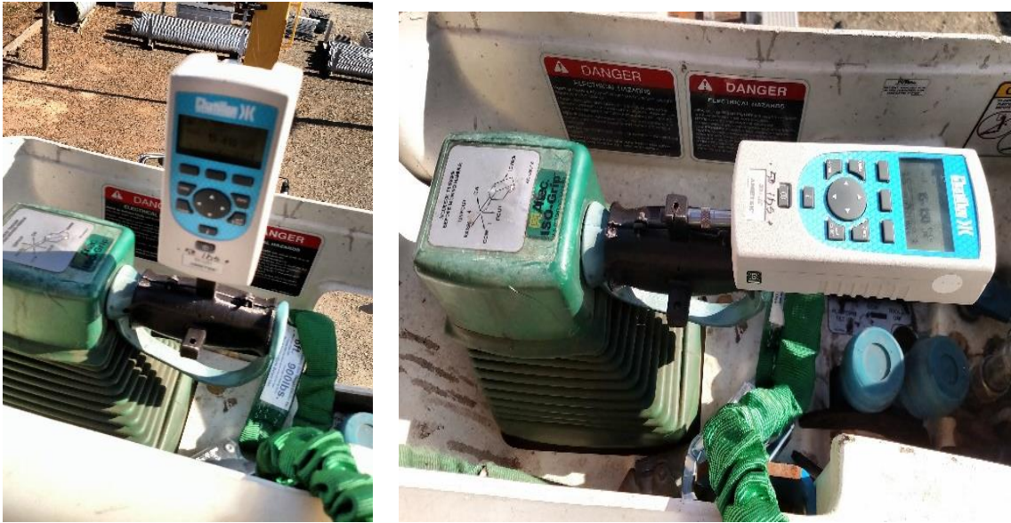
Figure 7. Chatillon force measuring setup for field study 2016. Same setup was used to test force for reduced force pistol grip in the laboratory. Measuring force for up/down direction (left). Measuring force for forward/rearward movement (right).
