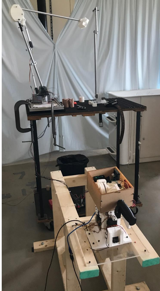
Figure 14. Laboratory setup of the 1/15th scale model bucket truck with power line and pistol grip mounted to laboratory test stand.
