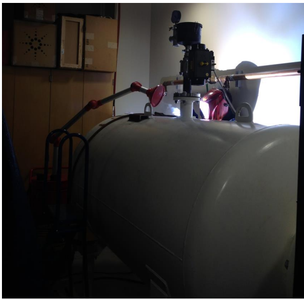
Figure 2.19 The catch tank: attaching the vacuum mount plate.
