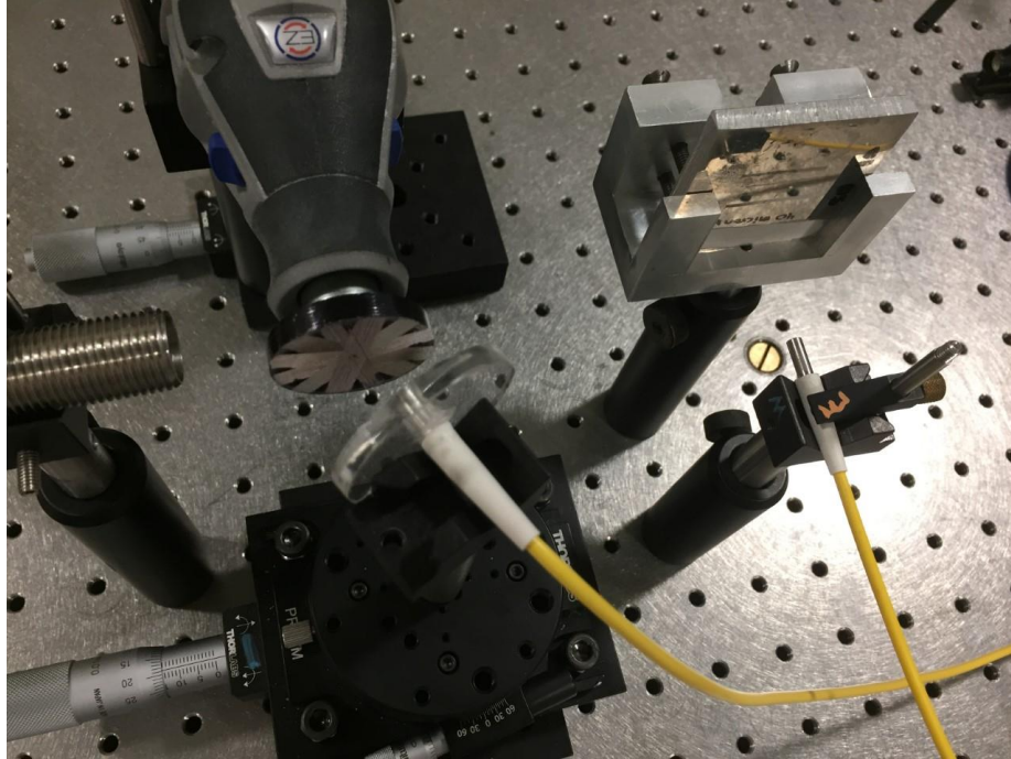
Figure 1.40 Optical PDV setup with yellow collimators testing moving targets (spun on the Dremel) and stationary targets such as the rectangular clamped sample.
