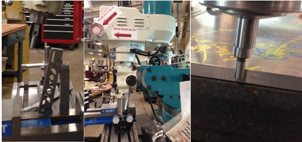
Figure 2.62 A myriad of tools are available to achieve higher precision machining. gauge blocks (mill), dials (mill and lathe) and the wiggler (mill) are all excellent tools to keep the dimensions of one's part on point.
