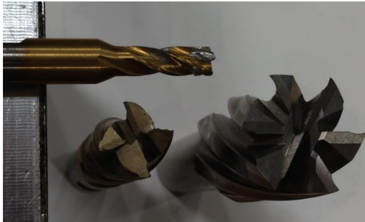
Figure 2.61 Examples of available milling tools from left to right, chipped teeth, clogged flutes, ideal tool.
