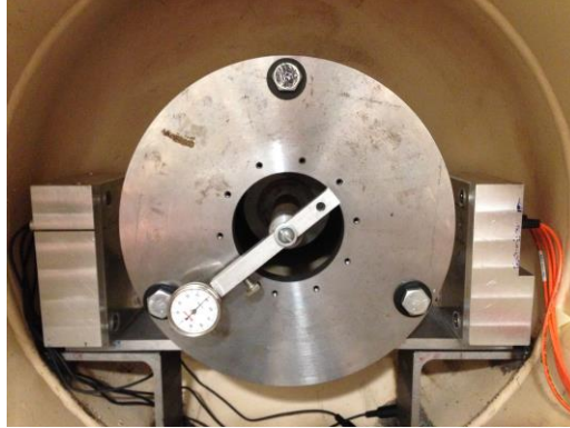
Figure 2.16 Dial indicator to align the target plate and a mounted sample.
