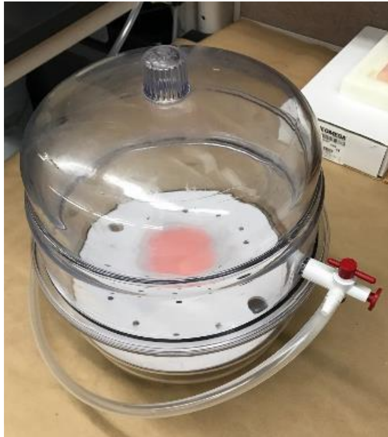
Figure 9: Vacuum chamber (Bel-Art Scienceware Desiccator) used to remove air bubbles after mixing the silicone base and activator.
