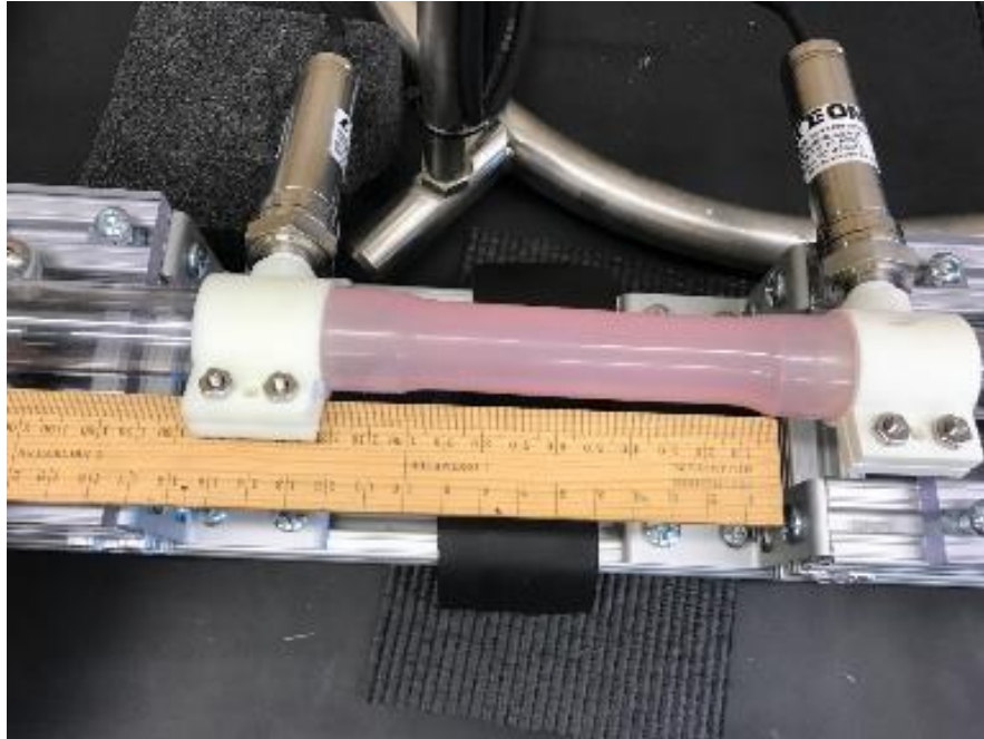
Figure 19: A ruler was used to measure longitudinal stretching.
