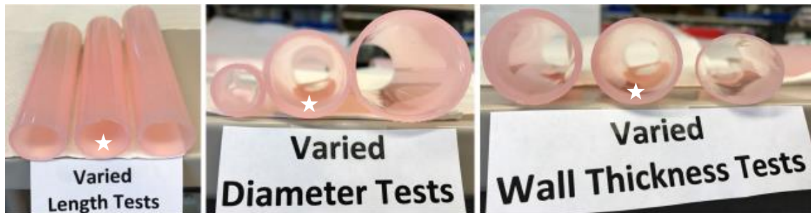
Figure 15: Comparisons of each tube geometry (length, diameter, and wall thickness). (★) Indicates the standard dimension tube ( L = 10\text{cm} , D = 22.22\text{mm} , W = 1.60\text{mm} ) for easier comparison with the varied dimensions in each study.
