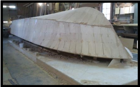
Figure 28 Full Size Custom Center Console Boat Under Construction
