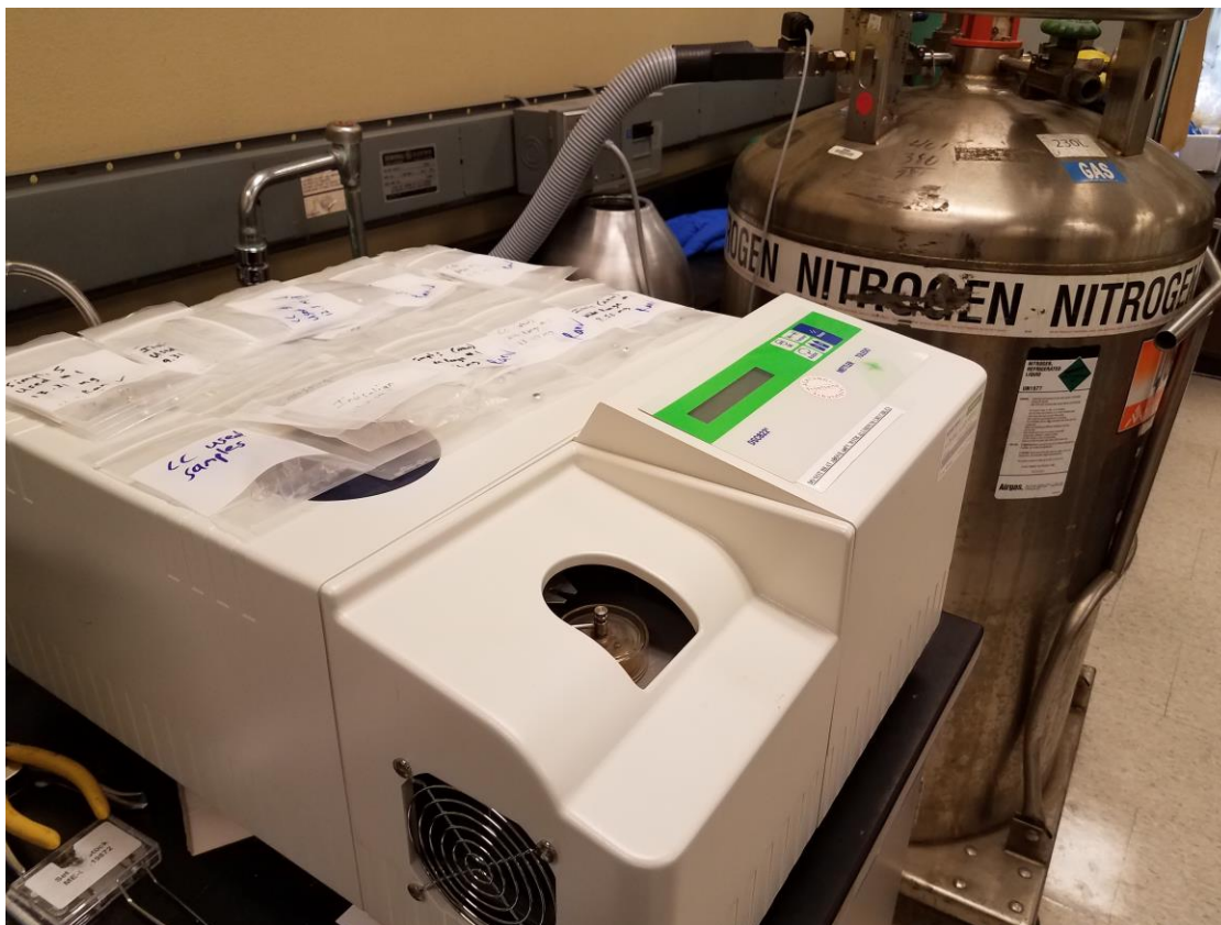
Figure 4: Mettler Toledo Model 822 DSC instrument with liquid nitrogen in the background used for thermoregulation
