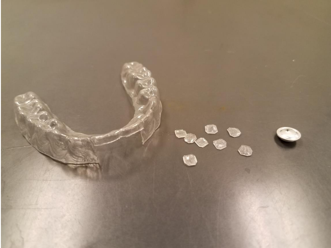
Figure 3: As-received Simpli5 aligner with a section removed for sampling, cut samples, and a prepared and sealed aluminum crucible ready for testing
