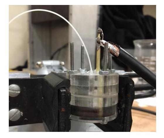
Figure 77: Target for the second shot featuring one collimator and one PZT pin.
