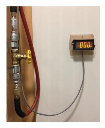
Figure 50: Dwyer DPMA-401 LCD screen with a pressure control valve.
