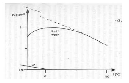
Figure 10: Density versus temperature for water in the solid line [19]
