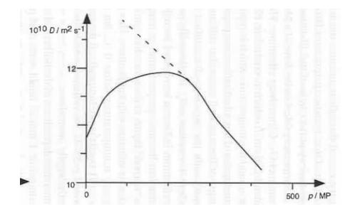
Figure 13: Diffusivity versus pressure for liquid water [10]
