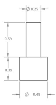
Figure 27: The projectile flyer made from copper, aluminum, or PMMA. Here all dimensions are in inches.
