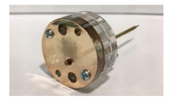
Figure 34: A sample after being sputter coated for two minutes.
