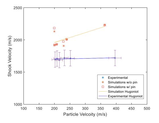
Figure 70: Experimental and simulated results displayed with error bars
