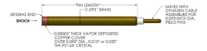
Figure 53: Piezoelectric Pin [19]
