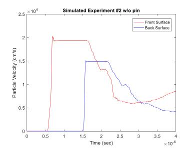
Figure 72: Simulated Results without a PZT pin in the design.
