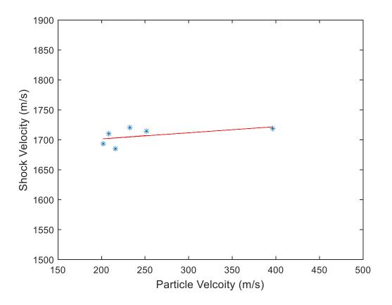
Figure 66: Experimental Results of the small gas gun experiment conducted at Marquette University.
