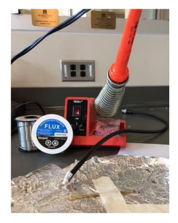
Figure 54: Soldering set up for connecting a BNC cable to a PZT pin.
