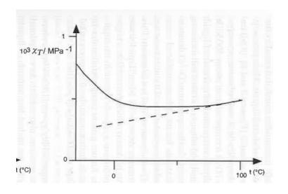
Figure 11: Isothermal compressibility, X<sub>T</sub>, versus temperature, t [10]
