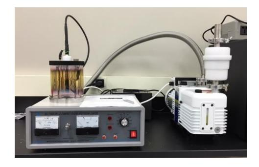
Figure 32: MTI Corporation model GSL-1100X-SPC12-LD sputter coating machine located in Marquette University Dental Research Laboratory
