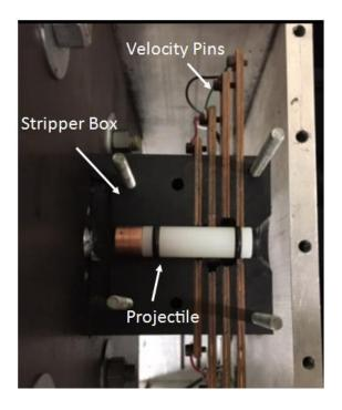
Figure 24: Stripper box, velocity break pins, and projectile
