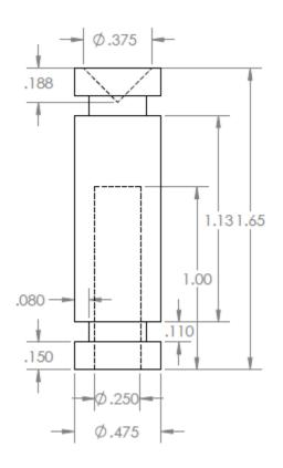
Figure 26: CAD drawing of the sabot design with all dimensions in inches.
