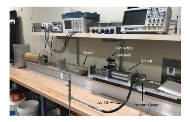
Figure 25: Overview picture of the equipment on the small gas gun
