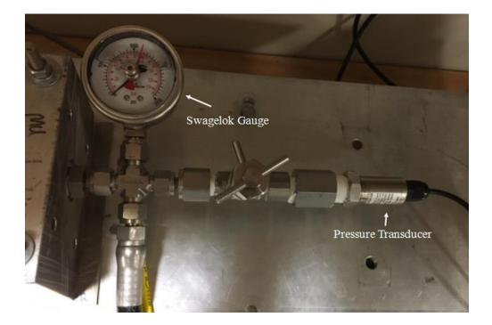
Figure 51: Swagelok gage and Dwyer pressure transducer
