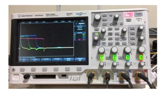
Figure 52: Agilent Technologies DOS-X-3034A oscilloscope with an output from velocity break pins
