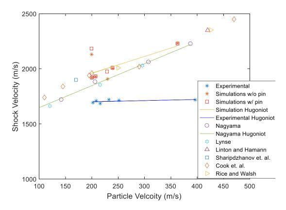
Figure 74: Experimental Results of the small gas gun experiment conducted at Marquette University compared to published data.
