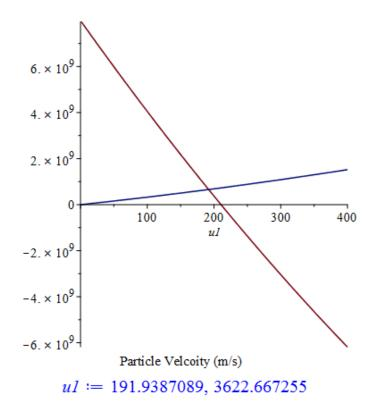
Figure 64: Particle Velocity versus Pressure for the flyer and driver interface.
