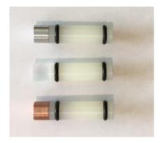
Figure 29: Nylon sabots with two O-Rings and flyers inserted
