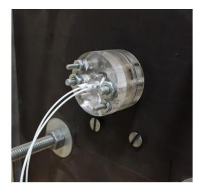
Figure 75: Original target sample with two PDV collimators exiting the design mounted onto the target plate.
