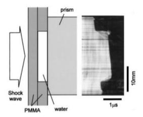
Figure 4: Experimental image used to determine the shock velocity by Nagayama [4].
