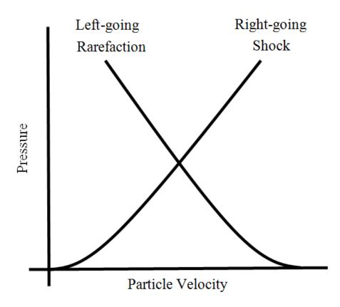
Figure 17: Demonstration of a left and right going wave in pressure-particle velocity space.
