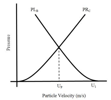
Figure 20: Left and right going waves in the pressure-particle velocity space for target pieces B and C.
