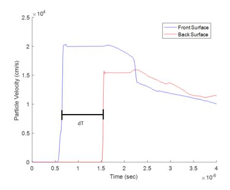
Figure 68:Simulated results used to find the wave traveling time.
