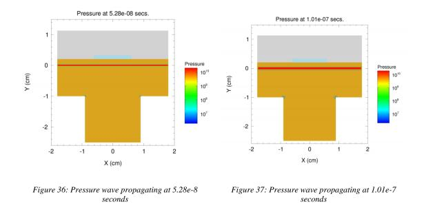
The shock wave begins to propagate through the material represented by the red line in Figure 36 where the flyer and driver come into contact. In Figure 37, one can see the rarefaction wave that is formed from the impact.
