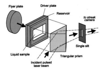
Figure 3: Experimental set up [4].
