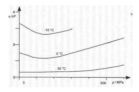
Figure 12: Viscosity versus pressure of liquid water at three fixed temperatures [10].
