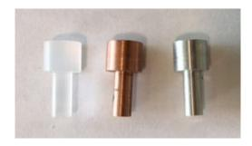
Figure 28: Physical flyers made from (left to right) PMMA, aluminum, and copper
