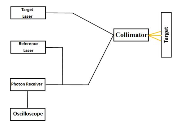
Figure 56: Schematic of the Photon Doppler velocimeter (PDV) at Marquette University.
