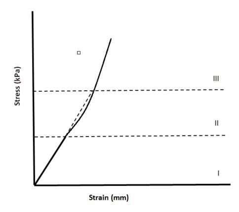
Figure 15: Typical stress versus strain graph with the three zones labeled
