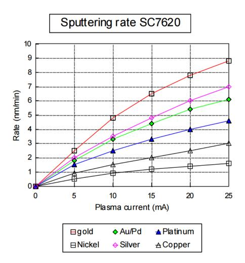
Figure 33: Graph for determining thickness of the gold sputter coating [18].
