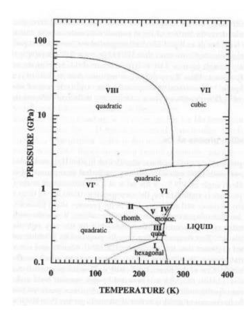
Figure 9: Pressure (GPA) versus temperature (k) of the ice forms [19]
