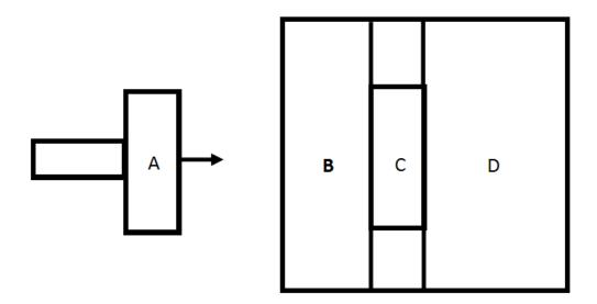
Figure 18: Schematic showing the flyer, A, and target, B, C, and D
