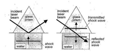
Figure 2: Demonstration of the experimental analysis for Mori et. al [2].
