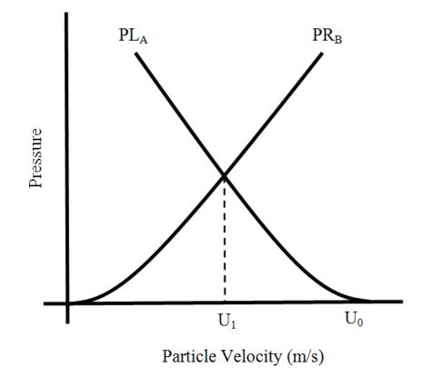
Figure 19: Left and right going waves in the pressure-particle velocity space for target pieces A and B.
