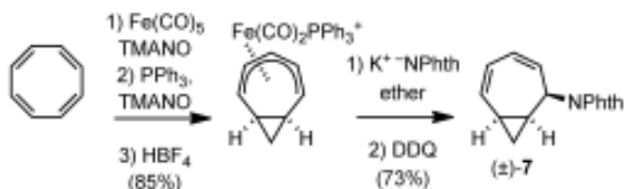
Scheme 1. Preparation of N -(bicyclo[5.1.0]octa-3,5-dien-2-yl)phthalimide 7 (TMANO=trimethylamine N -oxide).
