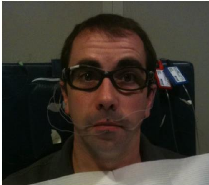
Figure 4- Subject with sensors attached to the tongue and lips and a reference sensor on the bridge of the glasses [2]
