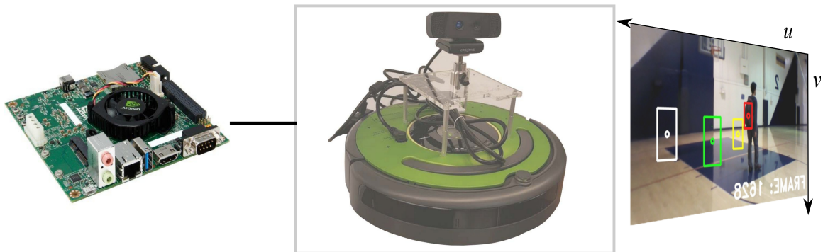
Figure 3.1: Overall system comprising an iRobot Create 2 platform with a Jetson TK1 board and a Creative Sens3D ToF camera.
