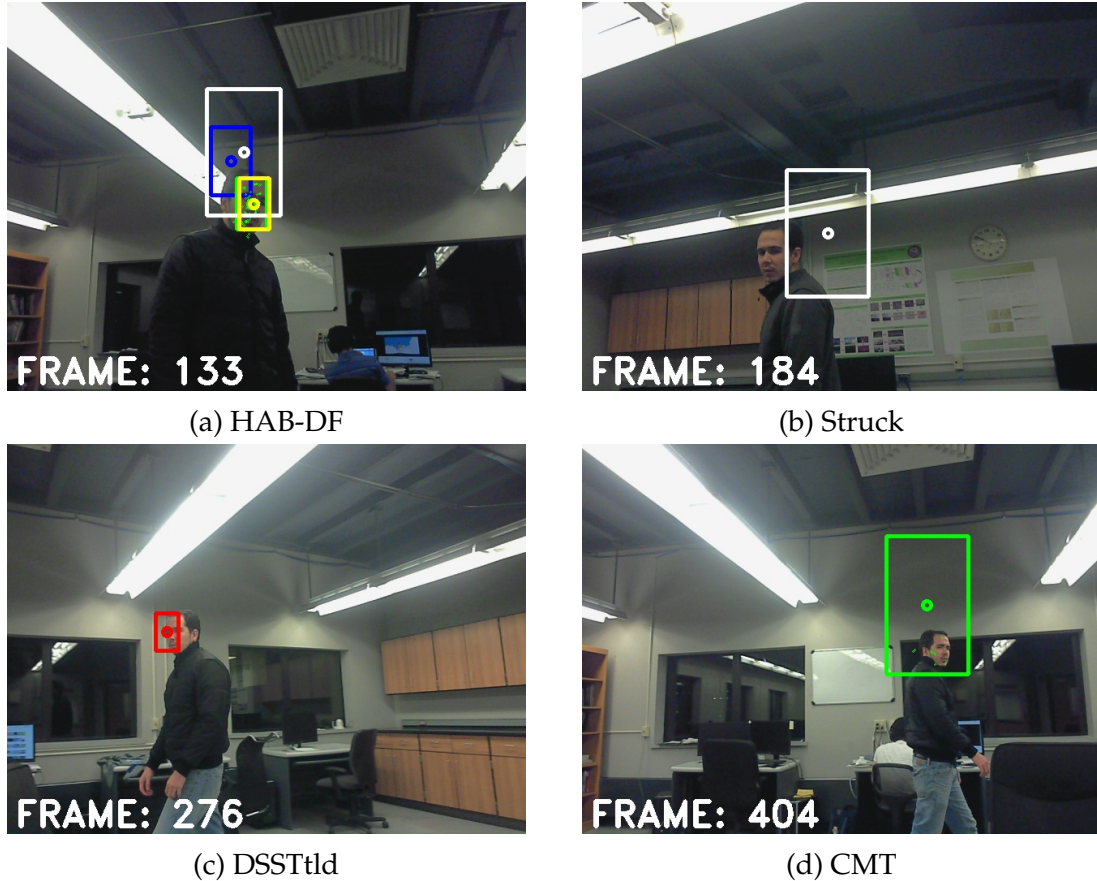
Figure 4.7: Pan-tilt system experiment using a face as the target (best seen in colors). The frames shown here are random frames selected from the dataset. Each of them presents a different tracking approach. The target was moving sideways with some vertical disturbances and gradually increasing the distance from the camera. In (a) HAB-DF is shown in yellow and DDSTtld is shown in blue because it is lost.
