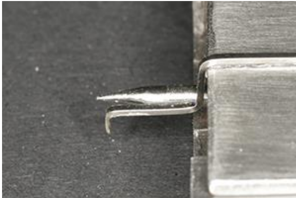
Fig. 3B. Wire adjusted to 0.3 mm thickness and placed on protective plate.
