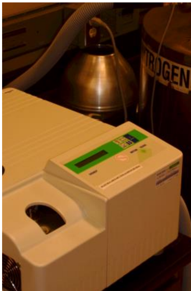
Figure 4: Mettler Model 822 used to conduct DSC analysis with Liquid Nitrogen as cooling agent
