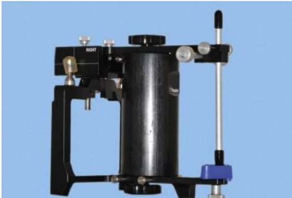
Figure 6. CPI-III used for assessing differences between Pana-Mount Facebow and Kois Dental Facial Analyzer System mounted casts.
