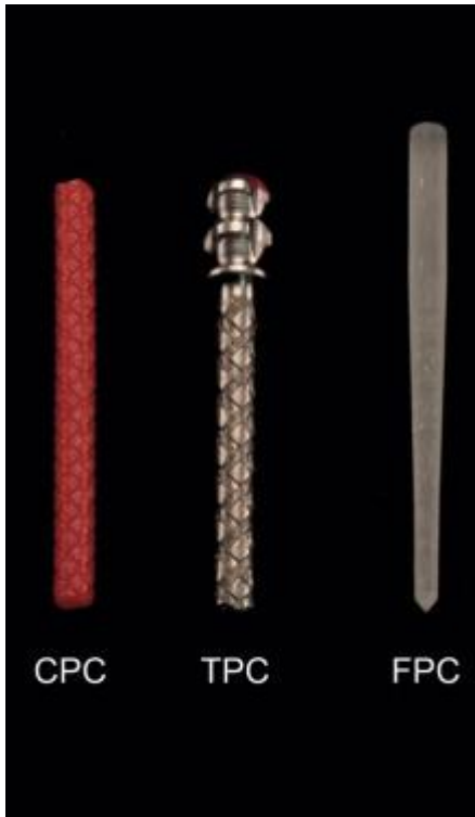
Figure 1. Photograph of 3 different post systems tested. CPC, Parapost XP-Lab (plastic pattern for custom cast post and core); TPC, Parapost XH (prefabricated titanium post); FPC, D.T. Light-Post (prefabricated quartz fiber post).
