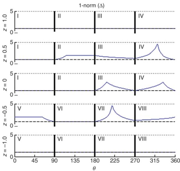
**Fig. 2** Stability boundary for third-order system with perturbations
