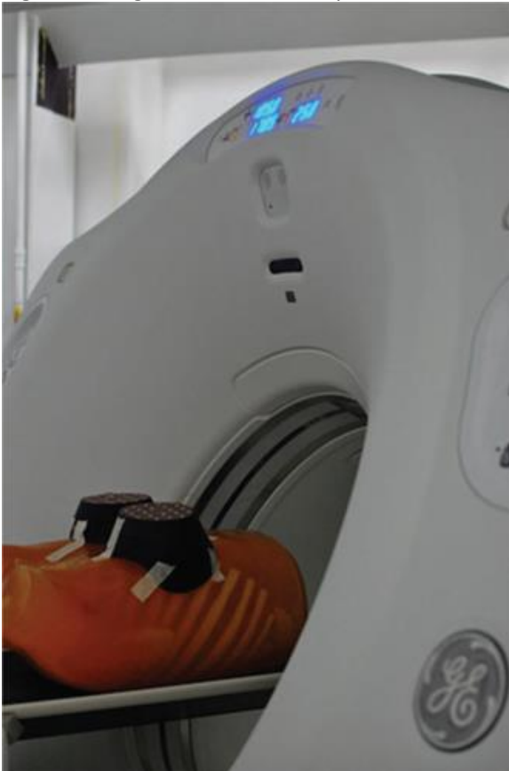
Figure 2 The GE CT750HD with its gantry tilted to perform a tilted acquisition.
