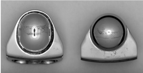
Figure 5. Micrograph of the superior (left) and inferior (right) endplates of a Prestige retrieved implant (2.3 years in vivo) showing a typical wear scar.
