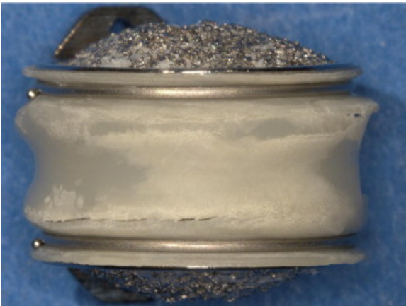
Figure 13. Posterior view of the sheath of a retrieved Bryan implant (1.6y in vivo ) showing the cloudy appearance along with areas of cracking. (Color version of figure is available online.)
