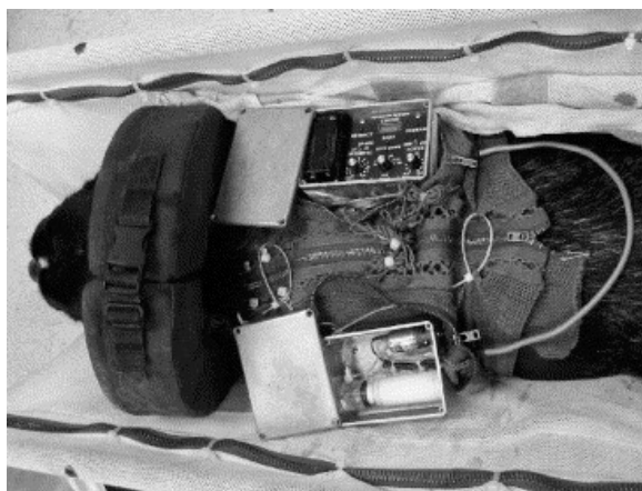
Fig. 4. Photograph depicting the aluminum boxes containing the electrical and mechanical components of the automated hydraulic coronary occlusion device stored in the jacket pockets of a typical conscious, chronically instrumented dog.
