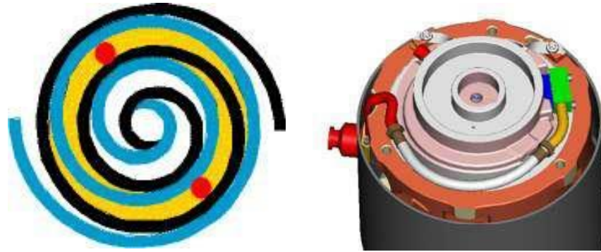
(a) Position of the Injection Ports in the Scroll Set
