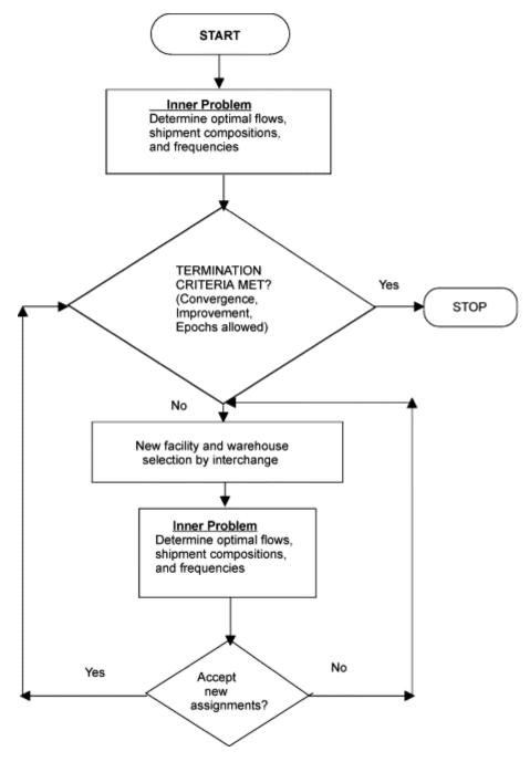
Fig. 2. Overview of simulated annealing.
