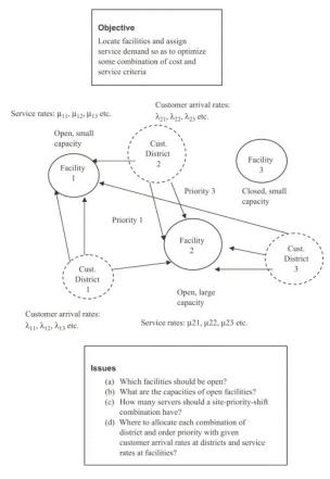
Fig. 1. Service system with multiple servers, order priority levels, and time shifts.
