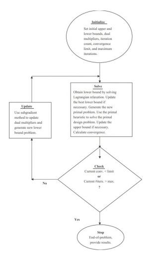
Fig. 3. Lagrangian methodology for system design.
