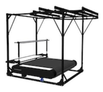
Figure 2. Blade skating treadmill with overhead gantry system. Adapted from [19].
