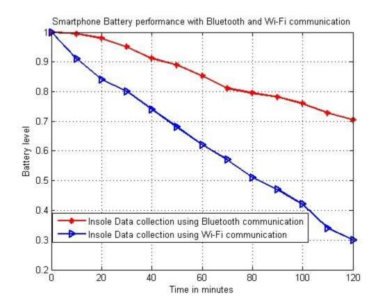
Figure 15. Blue curve presents the battery levels when the data collected using Wi-Fi communication and red curve presents the battery levels when data collected using Bluetooth communication
