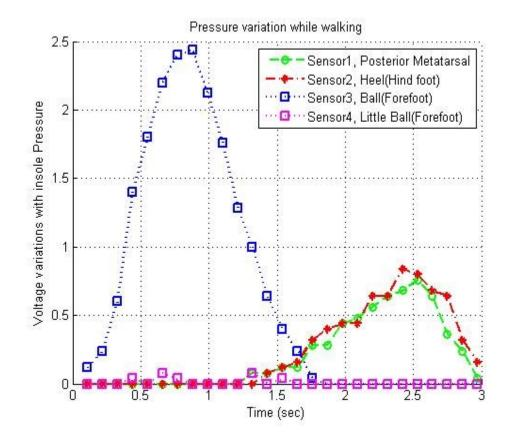
Figure 8. Insole Pressure Variation of an user while walking
