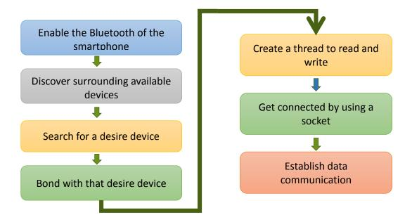
Figure 11. Algorithm on Smartphone for Bluetooth communication
