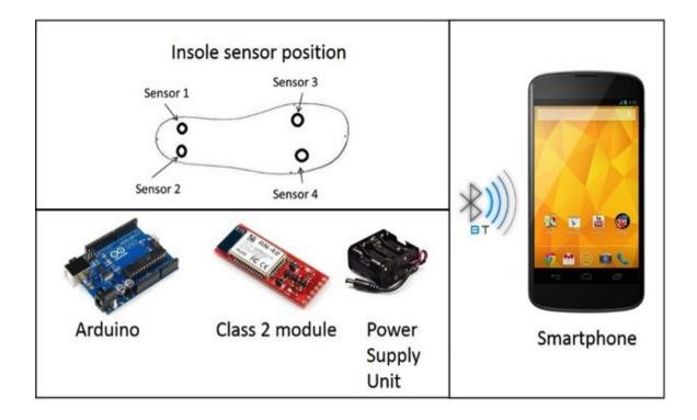
Figure 7. Components of a wireless shoe, and attachment sensors to the shoe with anatomical locations
