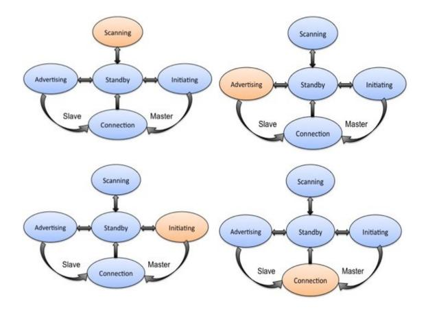
Figure 10. Different States of Bluetooth connection
