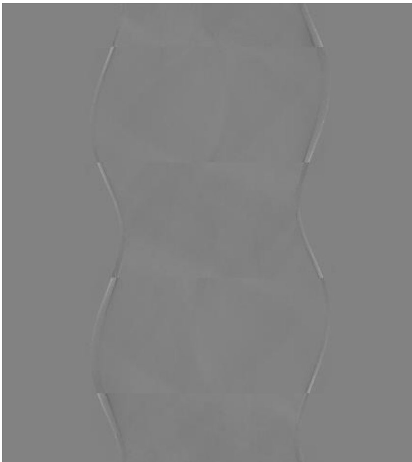
Fig. 27. A row of the pre-projection integration sinogram subtracted from the same row of the GPU-optimized sinogram. In this figure, the pre-projection integration version uses a software-based interpolation method instead of the hardware-based Texture Unit method. The histogram has been stretched to enhance the visualization of the error.
