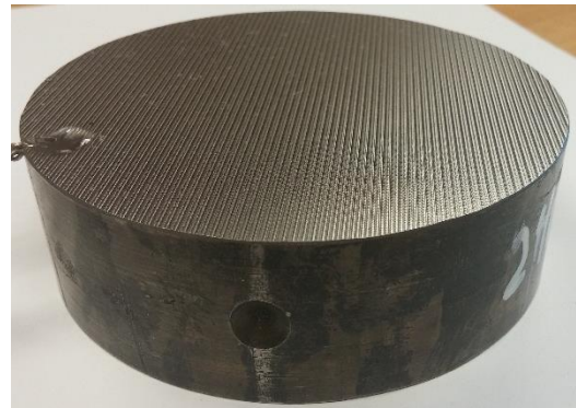
Figure 3.4 – Machined R_a 240 \mu\text{in} Platen Surface.
