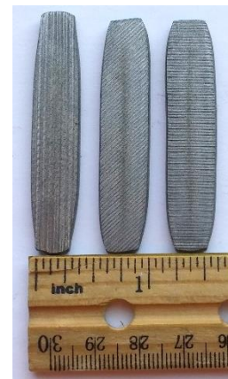
Figure 4.17f - Cigar compressed on R_a 240 \mu\text{in} , 300 °F platen using veg. oil lubricant.
