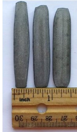
Figure 4.17b - Cigar compressed on R_a 20 \mu\text{in} , 300 °F platen using veg. oil lubricant.
