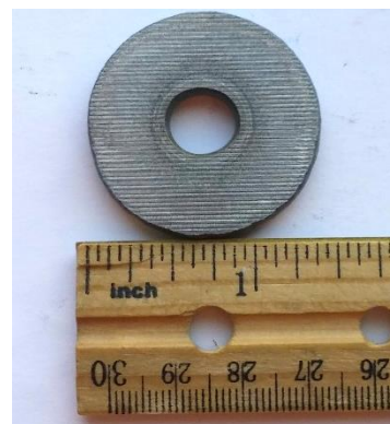
Figure 4.8c - Ring compressed on R_a 40 \mu in , 400 °F platen using veg. oil lubricant.
