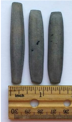
Figure 4.17a – Cigar compressed on R_a 10 \mu\text{in} , 300 °F platen using veg. oil lubricant.
