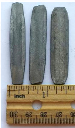
Figure 4.17d - Cigar compressed on R_a 60 \mu\text{in} , 300 °F platen using veg. oil lubricant.
