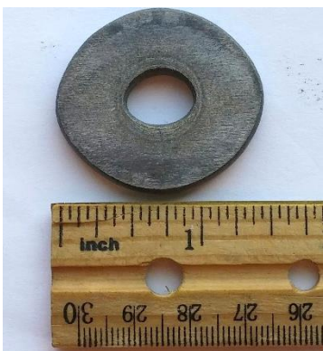
Figure 4.8a – Ring compressed on R_a 10 \mu in , 400 °F platen using veg. oil lubricant.
