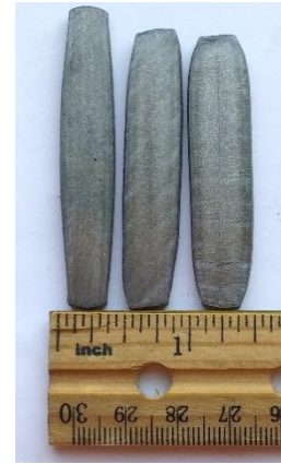
Figure 4.17c - Cigar compressed on R_a 40 \mu\text{in} , 300 °F platen using veg. oil lubricant.
