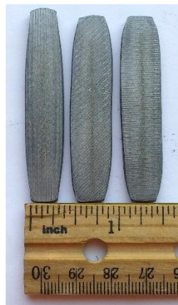
Figure 4.17e - Cigar compressed on R_a 130 \mu\text{in} , 300 °F platen using veg. oil lubricant.
