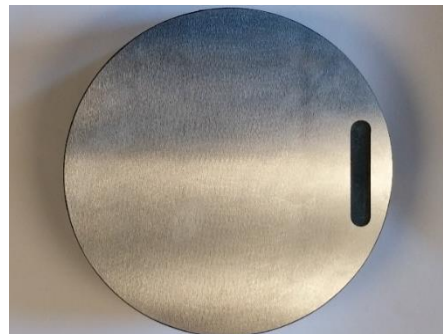
Figure 3.2 – Alignment groove on platen's working surface.
