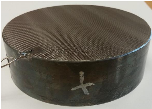
Figure 3.3 – Machined R_a 130 \mu\text{in} Platen Surface.
