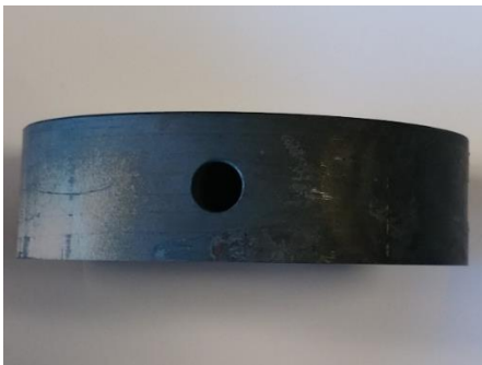
Figure 3.1 – Through hole drilled in platen's vertical face.
