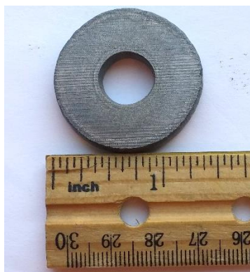
Figure 4.8b - Ring compressed on R_a 20 \mu in , 400 °F platen using veg. oil lubricant.
