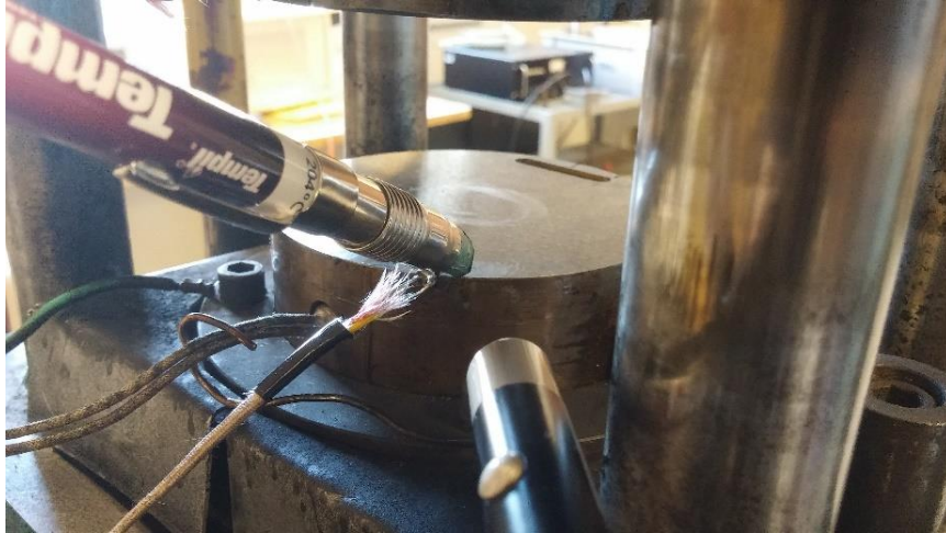
Figure 3.8 – Image of die temperature verification process.
