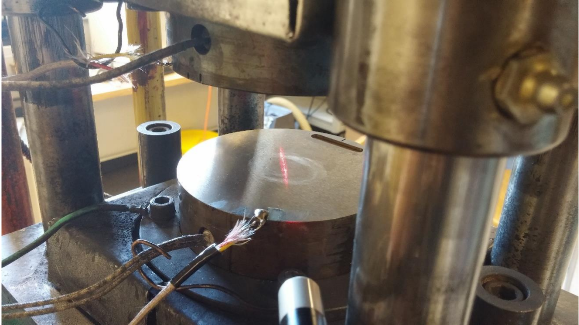
Figure 3.16 – Photo of the laser beam projected onto platen surface used to orient the cigar specimen
