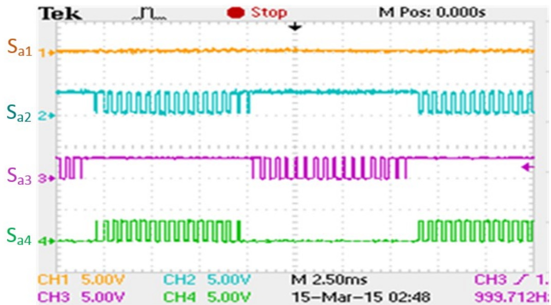
Figure 4.10: Measured PWM signals for the Phase-A leg of the three-phase three-level NPC inverter.
