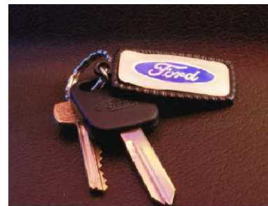
Figure 2.1.6 The new Ford keys containing RFID device to check the authenticity of the key
