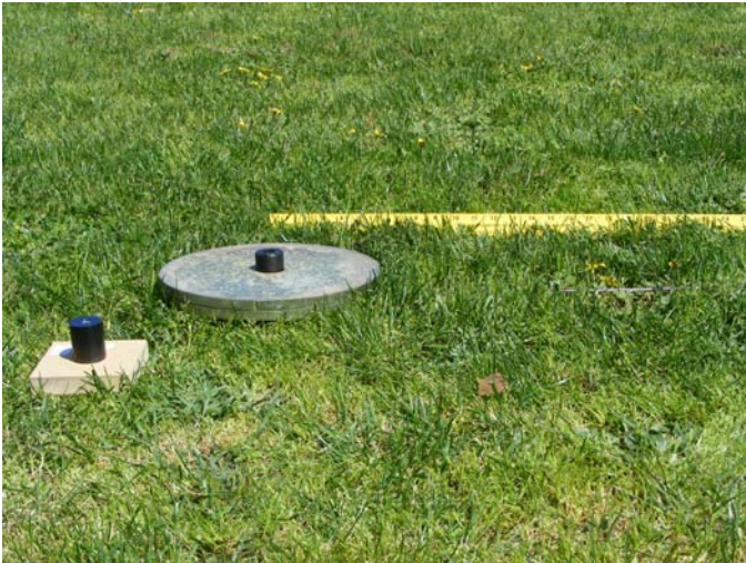
Fig 1. University of Ballarat device for measuring abrasion and surface friction.
