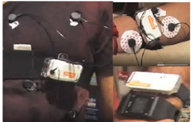
Figure 2. A patient wearing ECG in the chest, EMG in the forearm and a Accelerometer in the wrist.
