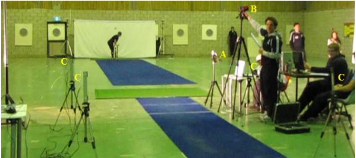
Figure 3.7. Experimental set-up of the pace bowling test. The high-speed camera (A), radar gun (B), and timing gates are shown (C).
