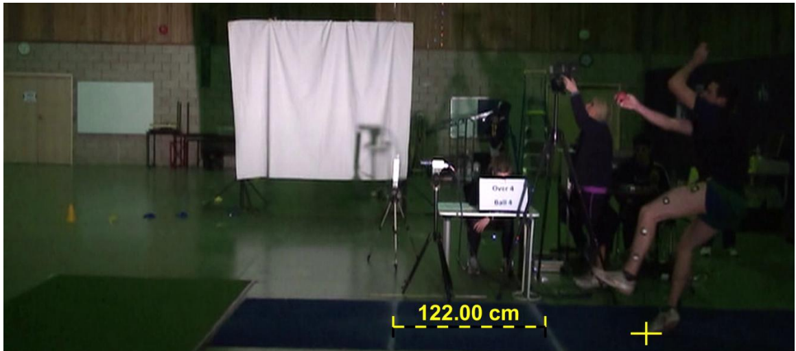
Figure 3.12. View from the digital high-definition video camera, with the white vinyl backdrop in the background. The distance between the bowling crease and popping crease (122 cm) was calibrated in Dartfish Connect so delivery step length could be estimated.
