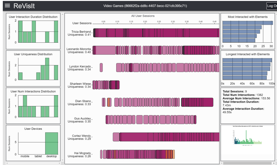
Figure 4.2: The ReVisIt dashboard includes an event timeline of user sessions in the middle, user and element summary charts on the side, key summary statistics, and an overlay visualization that shows the location of elements that users interacted with on the analyzed visualization.
