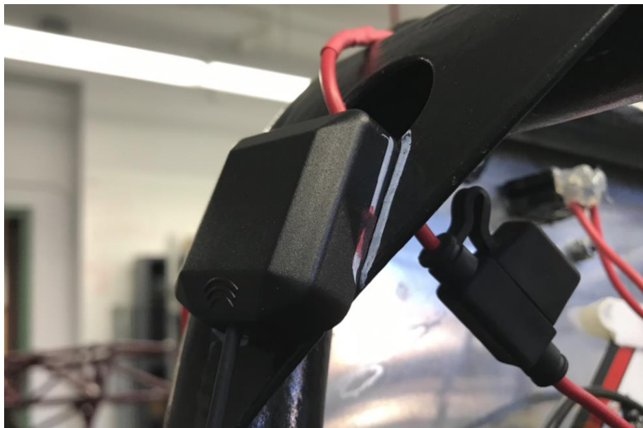
Figure 59. GPS Antenna Attached to Vehicle
