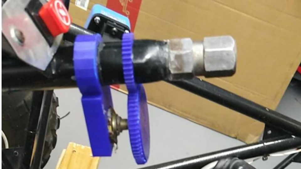
Figure 34. Potentiometer Cradle and Gears Printed and Mounted
