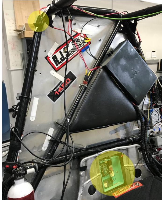
Figure 60. Baja Vehicle Highlighting Placement of GPS/IMU Box and GPS Antenna
