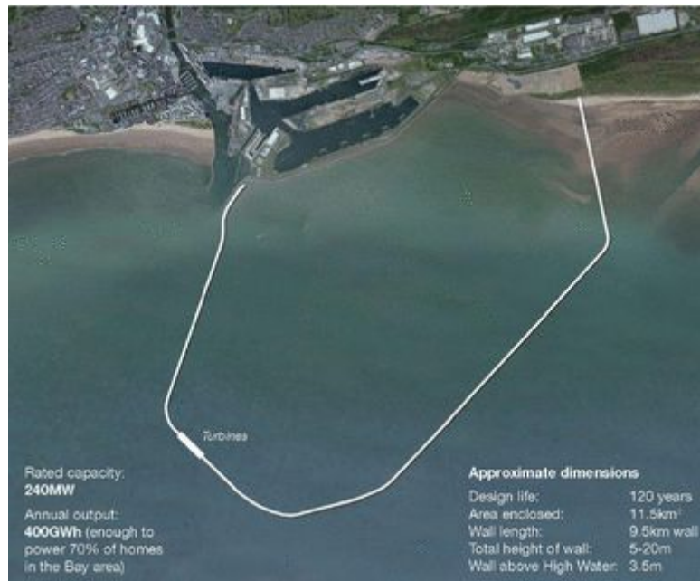
Figure 3.6 Proposed Swansea tidal lagoon. This site is not yet built only proposed. It artificially creates a reservoir to run the turbines instead of relying on natural reservoirs like a tidal barrage [9].
