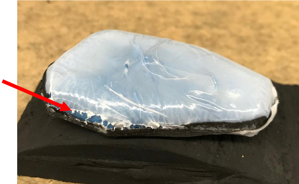
Figure 23. Polyethylene-encapsulated pad that burst after impact testing
