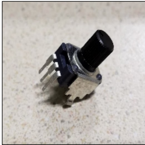
Figure 12 Potentiometer used for Passive RoboPuppet angle sensing.
