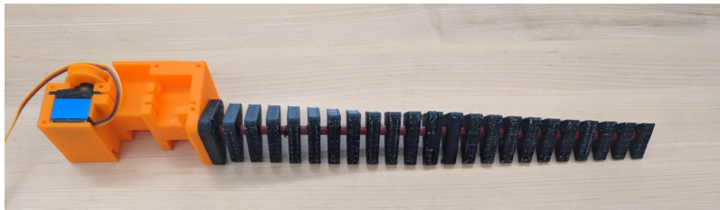
Figure 38: First full prototype of NinjaFlex tail
