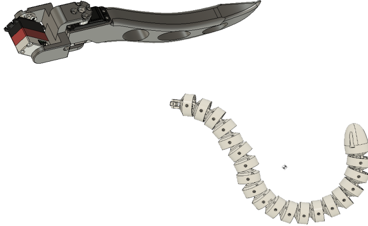
Figure 36: SmallKat's Solid Tail [Left] vs Continuum Tail [Right]
