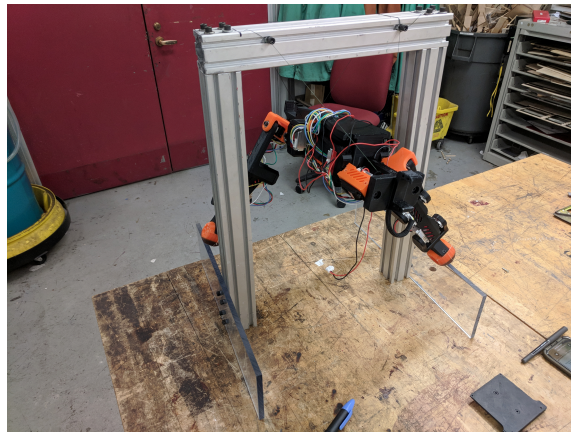
Figure 54: Prototype 6 up on a custom test jig designed to support the cat during testing
