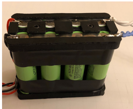
Figure 70: Custom Spot welded battery pack
