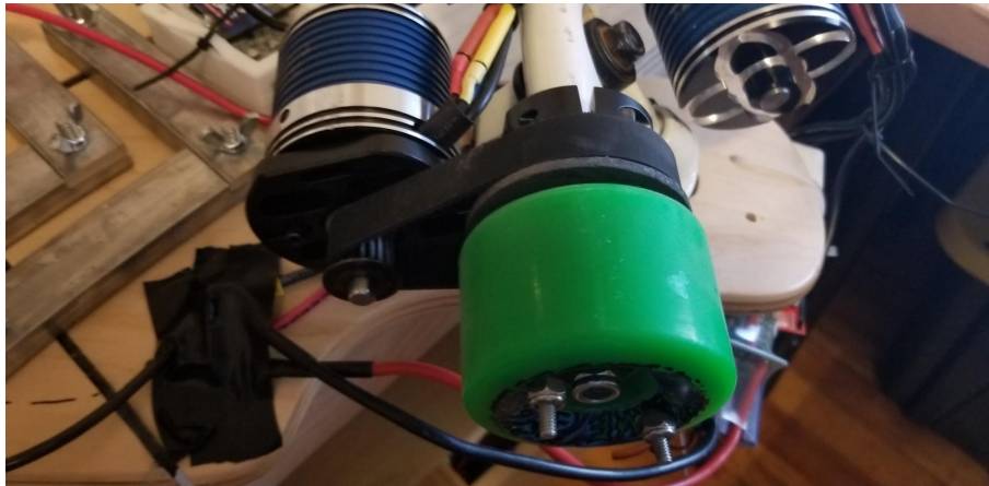
Figure 38: Motor Mounts with Motors on Board
