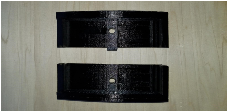
Figure 45a: Two halves of accessory housing after 3D printing
