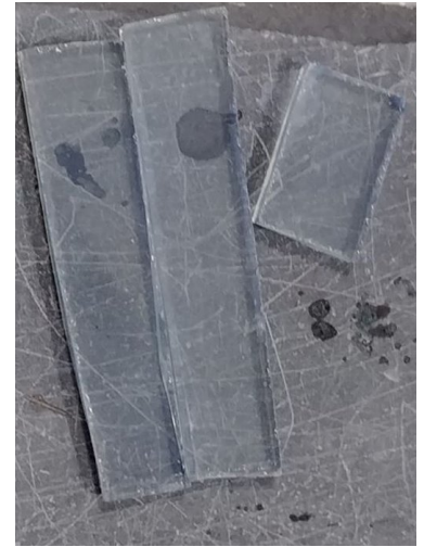
Figure 31: 1micron thick TiO 2 coated FTO glass.
