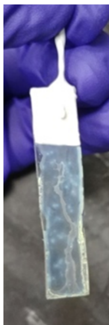
Figure 26: Electrode with 1 layer of WO_3 using dip-coating method. A 3.5 x 1 cm glass dipped into a 0.2M solution annealed at 550°C for 2 hours ramping for 4 hours with epoxy and wire attached for LSV/CA/Degradation testing.
