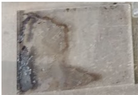
Figure 27: Cell with 1 burned layer of WO_3 + PEG using dip-coating method. A 3.5 x 3 cm glass dipped into a 0.2M solution annealed at 550°C for 2 hours ramping for 4 hours.
