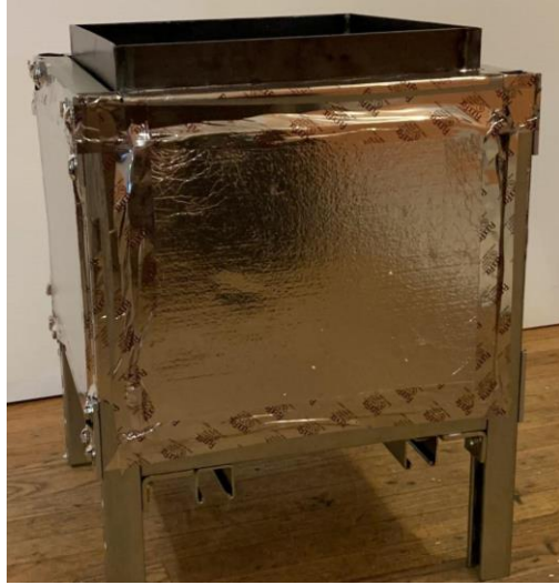
Figure A.5: Unit with a second layer of polystyrene and a layer of foil.
