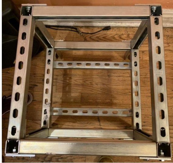
Figure A.2: The steel frame used to construct our custom refrigeration unit.
