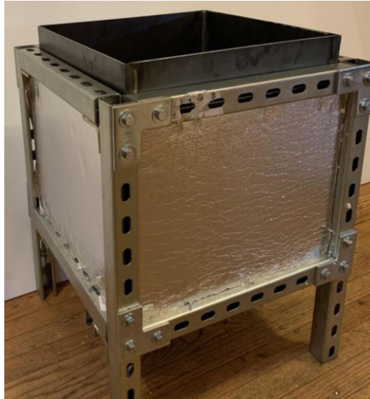
Figure A.4: Unit with polystyrene insulation added to surround the steel container.
