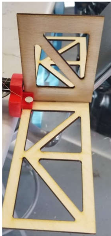
Figure 46. Structure of the vertical and horizontal tail used for glide testing
