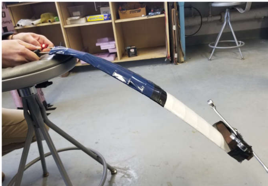
Figure 59. Full wing load test
