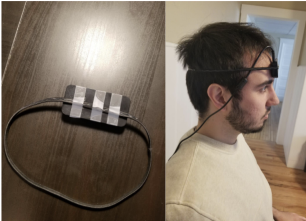
Figure 20: Headmountable Device (left) and Side Profile of user wearing device (right)
